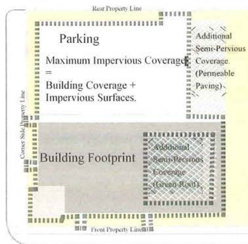
Figure 27-1811(a)-2. Maximum Impervious & Semi-Pervious Coverage.
