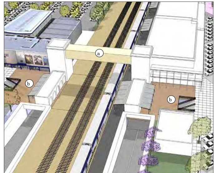
Figure 3.4 Conceptual model of pedestrian bridge as part of the Intermodal Transit Station discussed in detail in Section 3.3 (Public Transit). Concept includes placement and design of (a) a pedestrian bridge and (b) a pedestrian undercrossing.
