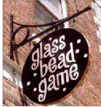
Projecting signs should fit within an imaginary rectangle with a maximum area of 12 square feet.
