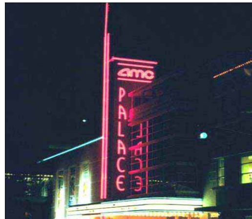
An example of internal illumination when the letters -- not the background -- are lit.
